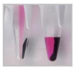
When removing supernatants it is important to remove as much of the liquid as possible without dislodging the particle pellet. With magnets used for manual protocols the particle pellet forms on the back wall of the sample tube. When placing the pipette tip inside the tube be sure to aim the end of the tip to the front wall of the sample tube to avoid disrupting the particle pellet.
